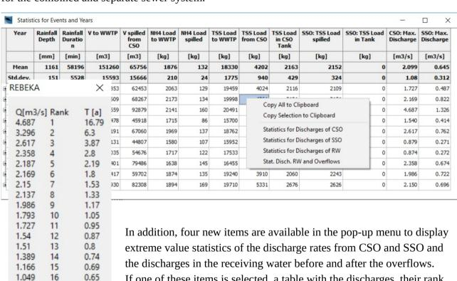
If one of these items is selected, a table with the discharges, their rank and annuality appears. This table is automatically copied to the clipboard and can be pasted with Ctrl-V, for example be inserted into a spreadsheet.
