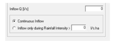
constant inflow should be active. If the rainfall intensity falls below this value, the inflow is 0. This makes the simulation of a throttle flow from an upstream CSO more realistic. Nevertheless, it is recommended to do the modeling with two separate projects (one for the upstream CSO and one for the following structure) and to use the throttling flow of the first project stored in a file as an inflow in the second project.
